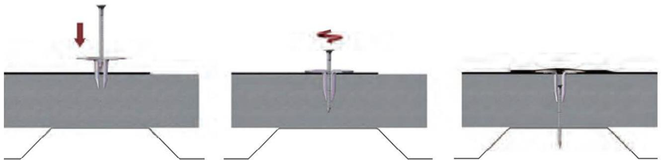
1. Lightly insert the washer and IKOfix Universal fastener into the insulation board.
