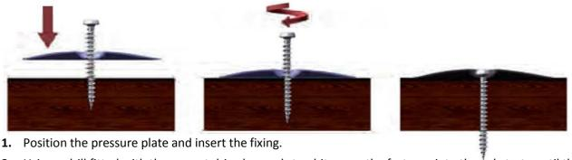
**2.** Using a drill fitted with the correct drive bar and stop bit screw the fastener into the substrate until the fixing depth is reached.
