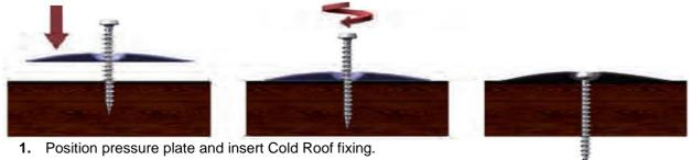
2. Using a drill fitted with the correct drive bar and stop bit screw the fastener into the substrate until the fixing depth is reached.
